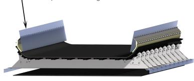
**SPARET** The EXP requires minimal maintenance. The inside skirt board seals are self-adjusting, and the slide rails have a lifespan of several years.
