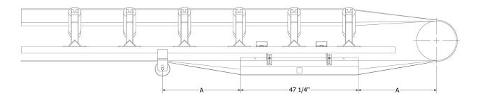
Detail - SPAR 7 location when the tail pulley is equipped with a SPAR 4 rock deflector
