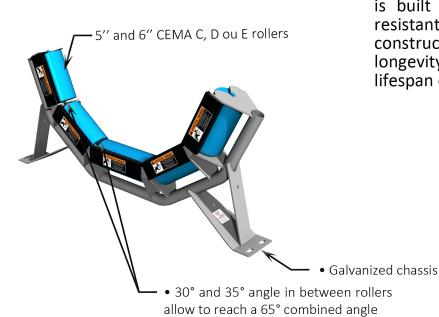
The MS SPAR deep troughing idler is built to last. The sturdy and resistant materials used in its construction guarantee its longevity, as well as extend the lifespan of your installations.
