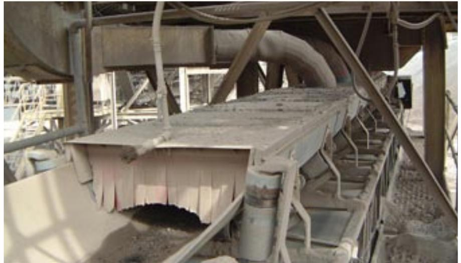
Transpar dust collector installed at the secondary crushing stage of the Montreal East quarry.
