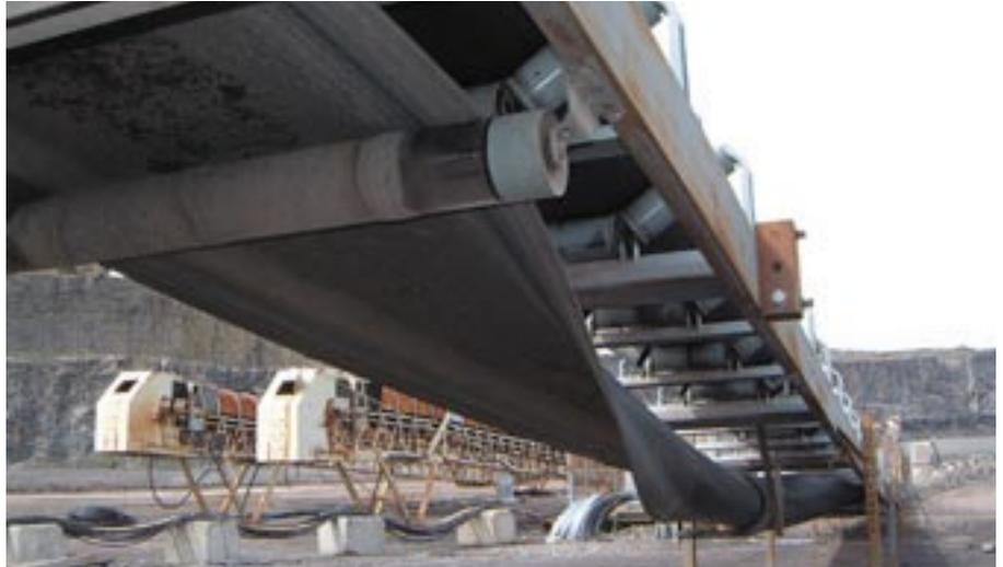
View of the belt turnover system installed on conveyor C-7 at Lafarge Canada's Montreal East quarry. The system has eliminated carryback spillage under the return idlers.
