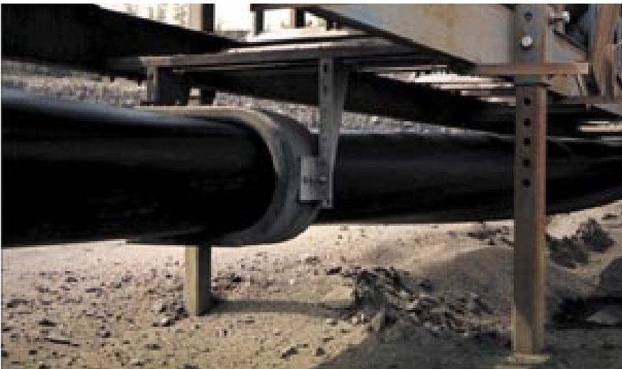
The SPAR 3 polymer guide smoothly flips the belt so that the driving side remains clean and dry.
